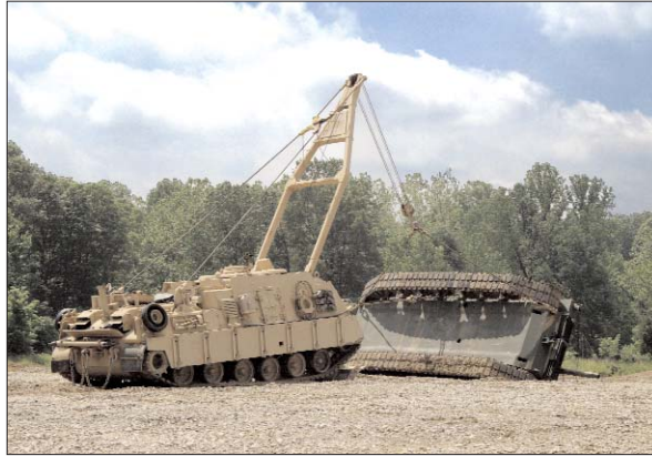
The M88A2 is a full-tracked, steel armored recovery vehicle that features increased hoisting, winching and towing capability for battlefield recovery of tanks and other similar vehicles.
