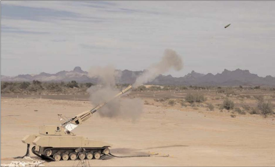
The Non-Line-Of-Sight (NLOS) Cannon fires its first round at an Army testing facility. The successful firing marked the first time a U.S. howitzer fired its very first live-fired round using tactical software. The NLOS Cannon is part of the Future Combat Systems (FCS) program.
