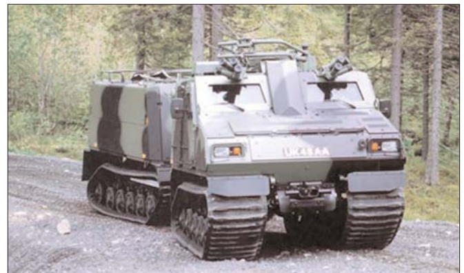
The BvS10 is a further development of the smaller Bv206S, with improved load capacity, based on the experience gained from more than 25 years of articulated vehicle design and production. BvS10 offers a load capacity of 3 to 5 tonnes.
