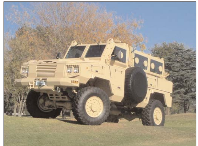
RG31 is the mine-protected vehicle of choice of peacekeepers. The all-steel, welded armour, monocoque hull protects the crew against AP rifle fire and anti-tank mine detonations. In standard APC configuration, this air-conditioned vehicle carries a crew of 10 (driver plus 9).
