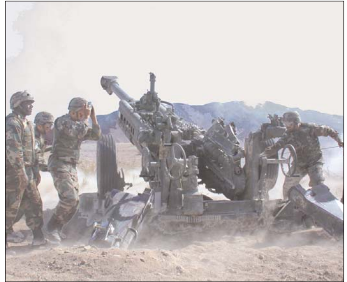
Highly mobile on land, at sea and in the air, the M777 has increased survivability. It is the world's first 155mm Howitzer weighing less than 10000 lbs .
